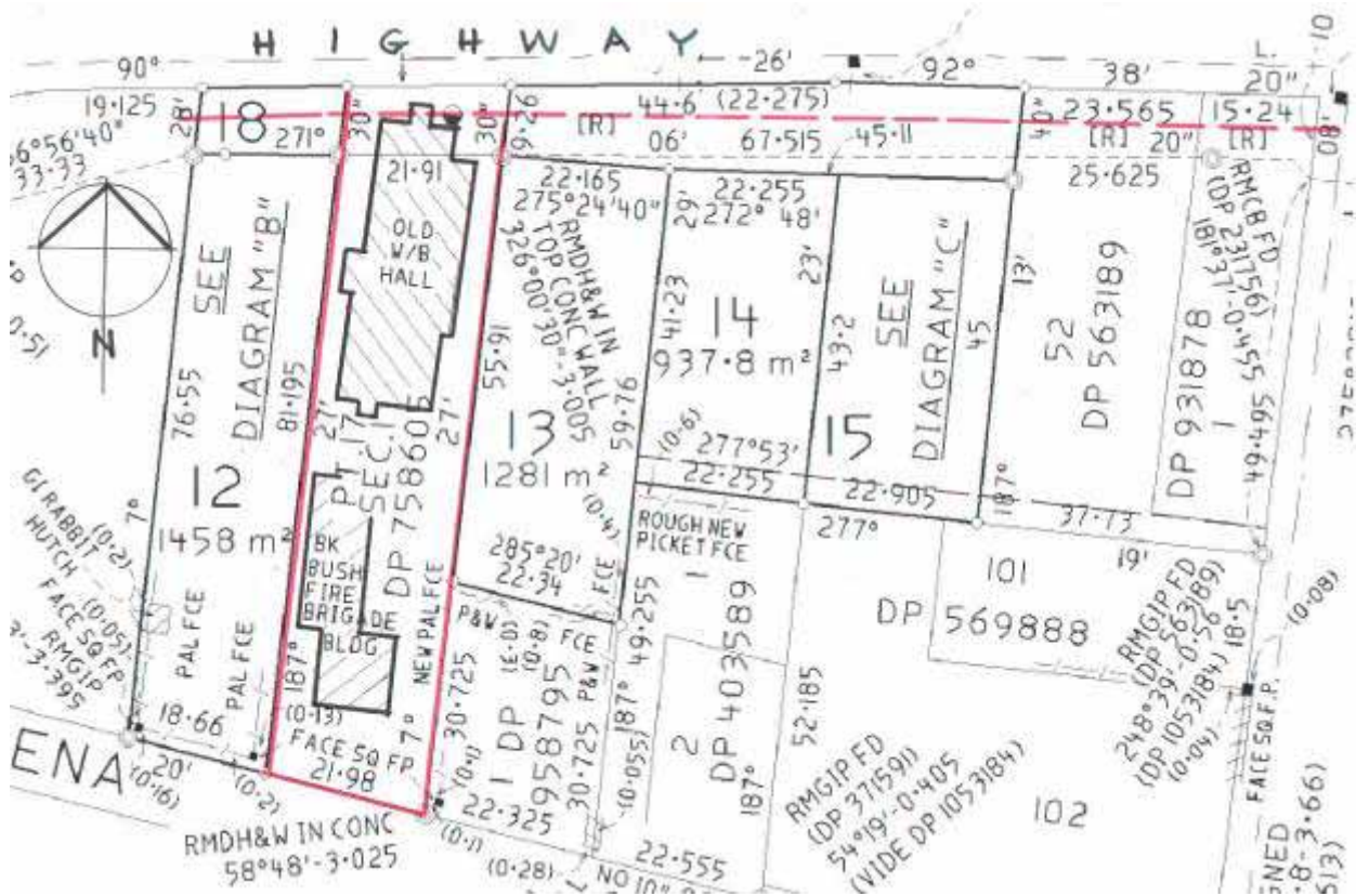
FIGURE 1: Location plan showing previous RTA highway widening and land acquisition (and possible new alignment in dashed red)
